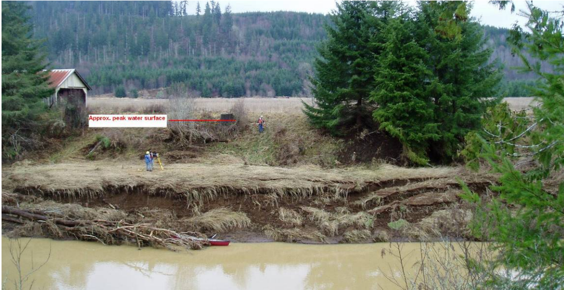
Figure 11. USGS photograph of the water surface for the Chehalis River near Doty. Source is USGS Press release of February 5, 2008: New Peak Flow Record for the Chehalis Flood. http://wa.water.usgs.gov/news/2008/news.chehalis.newpeak.htm
